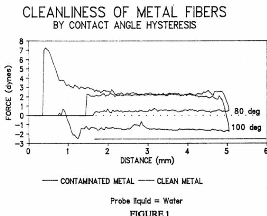
An overlay of a wettability scan with water shows an advancing contact angle for the clean metal wire of 80 degrees, as compared to a 100 degree advancing contact angle for the contaminated wire sample. Although both scans show a similar receding trace, the hysteresis between advancing and receding angles is significant.
