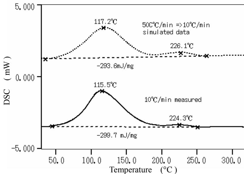
Figure 6 DSC Results for Epoxy Adhesives
