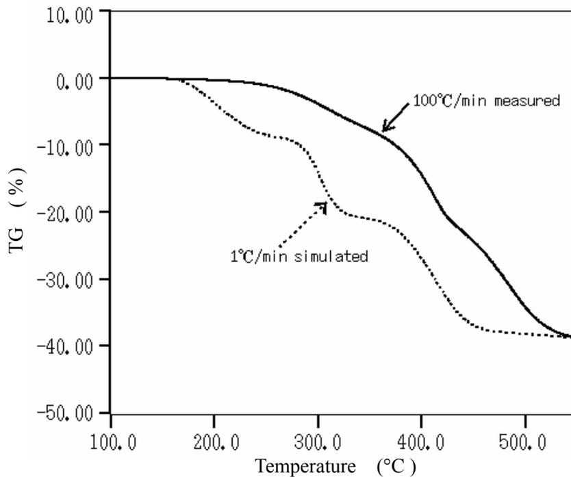
Figure 4 TG Results for Chloroprene Rubber
