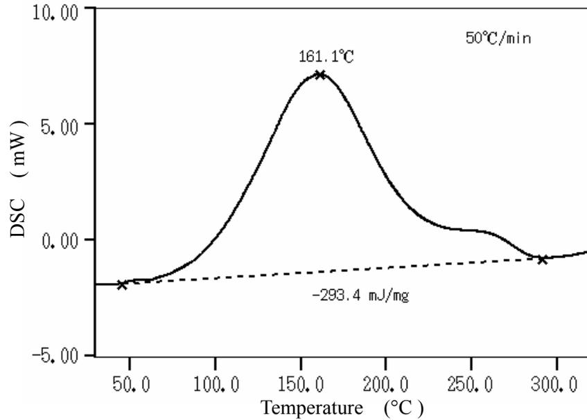
Figure 5 DSC Results for Epoxy Adhesives
