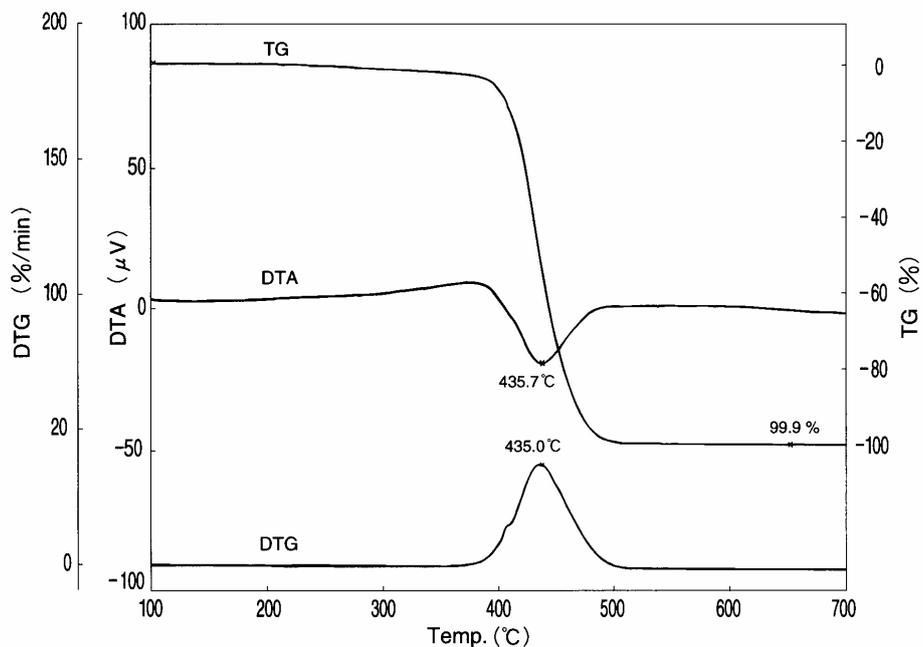
Figure 2 TG/DTA Measurement Results for ABS resin in N<sub>2</sub><sup>1)</sup>
