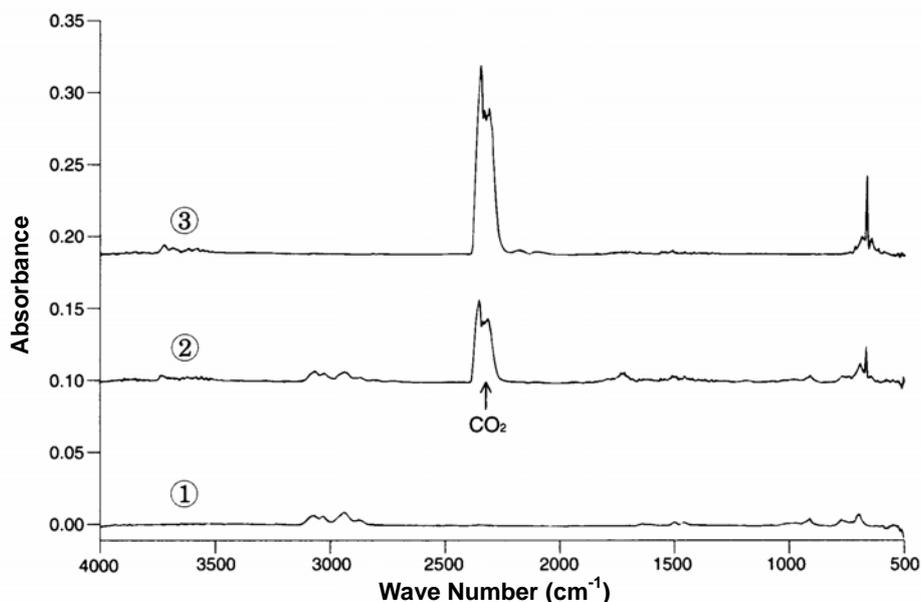
Figure 4 IR absorption spectrums of decomposition gas in air and N<sub>2</sub>
