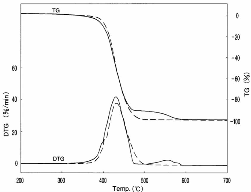
Figure 3 Comparisons of TG and DTG curves in air and N<sub>2</sub>
