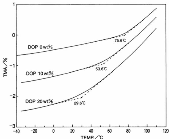
Figure 2 TMA Measurement Data for Each PVC Samples
