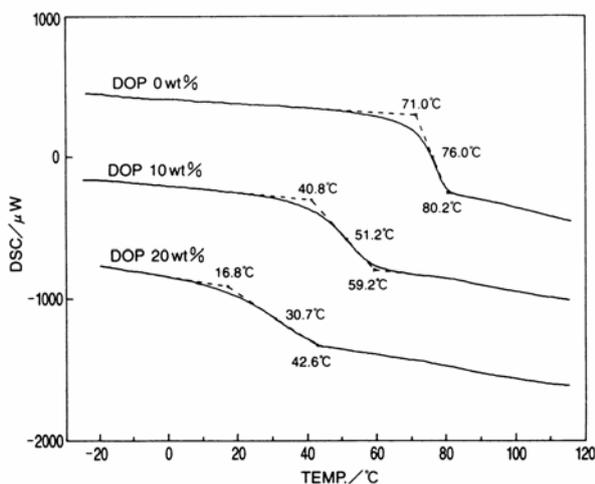
Figure 1 DSC Measurement Data for Each PVC Samples
