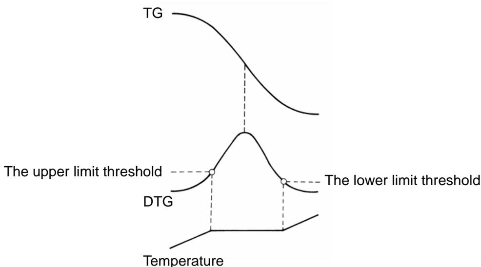
Figure 1 The Principles of Quasi-Isothermal Thermogravimetry<sup>5)</sup>
